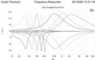
All diagrams on this double page show the filter characteristics of the analog RackPack Ranger modules. The lower bands have relatively narrow bandwidths for fundamental tones, the upper bands have broader bandwidths to process groups of overtones in common.
